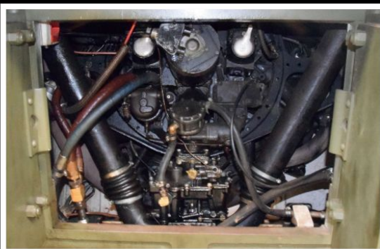
Above: The M3 Lee was powered by a Wright (Continental) R975 EC2 nine-cylinder air-cooled radial 400hp petrol engine.
